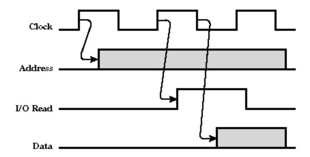
On the first clock signal, the port address is output to the address bus. On the second signal, the I/O Read line is activated, causing the selected port to place its data on the data bus. On the third clock signal, the CPU reads the data.
